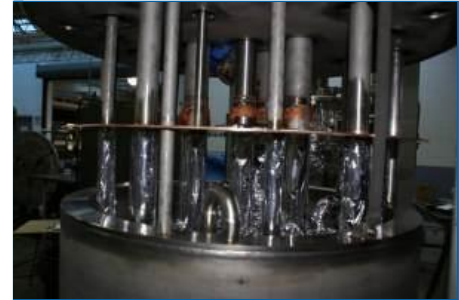
Thermoacoustic oscillations can develop in tubes which connect a cryogenic reservoir to room temperature.
