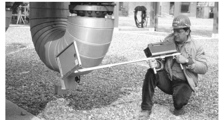
Fig. 10-18. Flash radiography of an insulated pipe section
