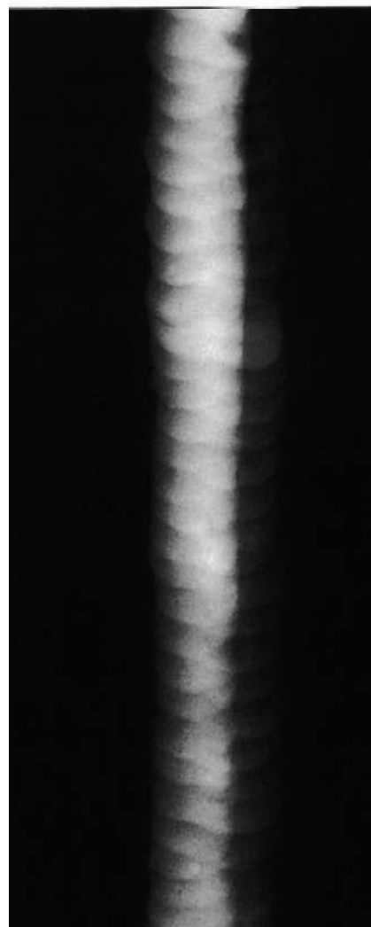
Offset or mismatch (Hi-Lo). An abrupt change in film density across the width of the weld image
