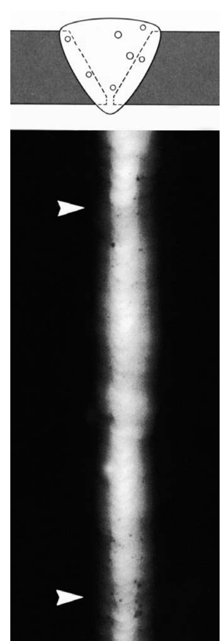
Scattered porosity. Rounded spots of darker densities random in size and location.
