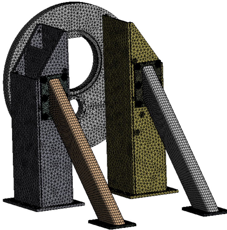
Figure 81. FE model of feedcap support
