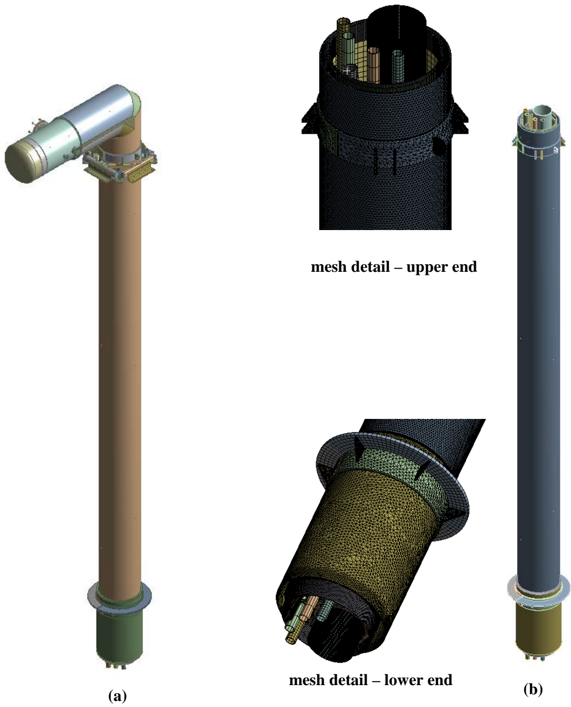
Figure 25. Finite element model of vertical anchor module
