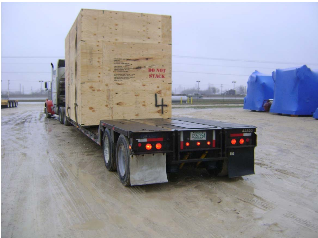
Figure 18: Process module crated for international shipping. Shrink-wrapped process modules can be seen in the background
